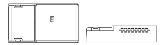
DR800-DL series LED driver, a family of DALI-2 & Push-DIM independent ECG covering from 3.5W to 57W, design with through wiring and super large wiring space, saving a lot of time and effort on the actual wiring work on site. Big push-fit looping connectors are quick to connect cables with, supporting also various wire thicknesses. Wires are secured to the driver with click-on cable clamps, and strain relief cover clicks on effortlessly securing the connections without any need for screws.
